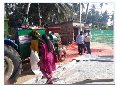
highly appreciated the machine as the commercially available axial flow thresher discharge the chopped straw which is of no use to them but this machine discharge the whole straw which can be used for mushroom cultivation in their area. The farmers expressed that by using this machine, they can get additional income of Rs 3500/- 4000/- per acre by selling straw bundles.
